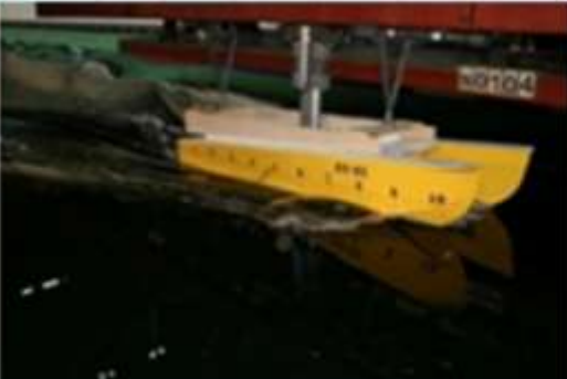
Tank Tests With Experimental Hull
